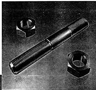
The rising sector gates of the Thames Barrier, downstream from the Port of London, are secured through hinge assemblies incorporating over 8,000 36mm diameter stud bolts in MONEL alloy K-500 and over 16,000 72mm diameter MONEL alloy 400 nuts and washers.
